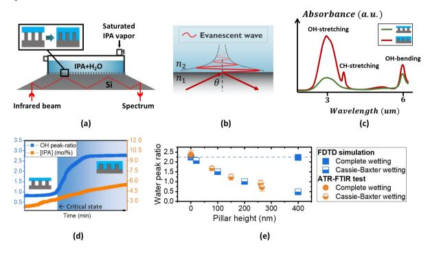
(a) Sketch of the ATR-FTIR-based wetting state characterization experiment set-up.
